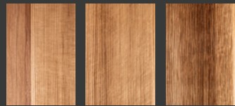
Wire Brush From Left to Right - Light, Medium, Heavy
