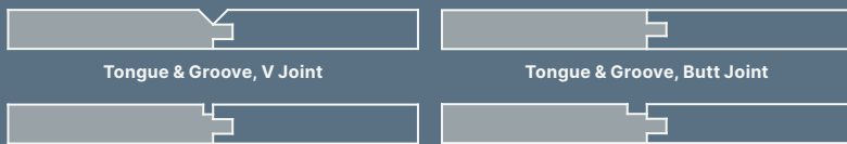
Tongue & Groove, Butt Joint w/ 1/8" w x 1/8" d Channel Groove
