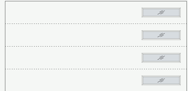
SW-17: Right Flush Side Windows, 4 Sections
